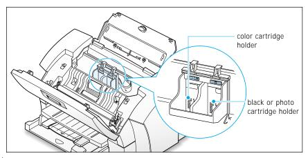
6. Holding the top handle, insert the color cartridge in the left holder, and insert the black (or photo) cartridge in the right holder. **Both cartridges must be installed for proper operation**.
